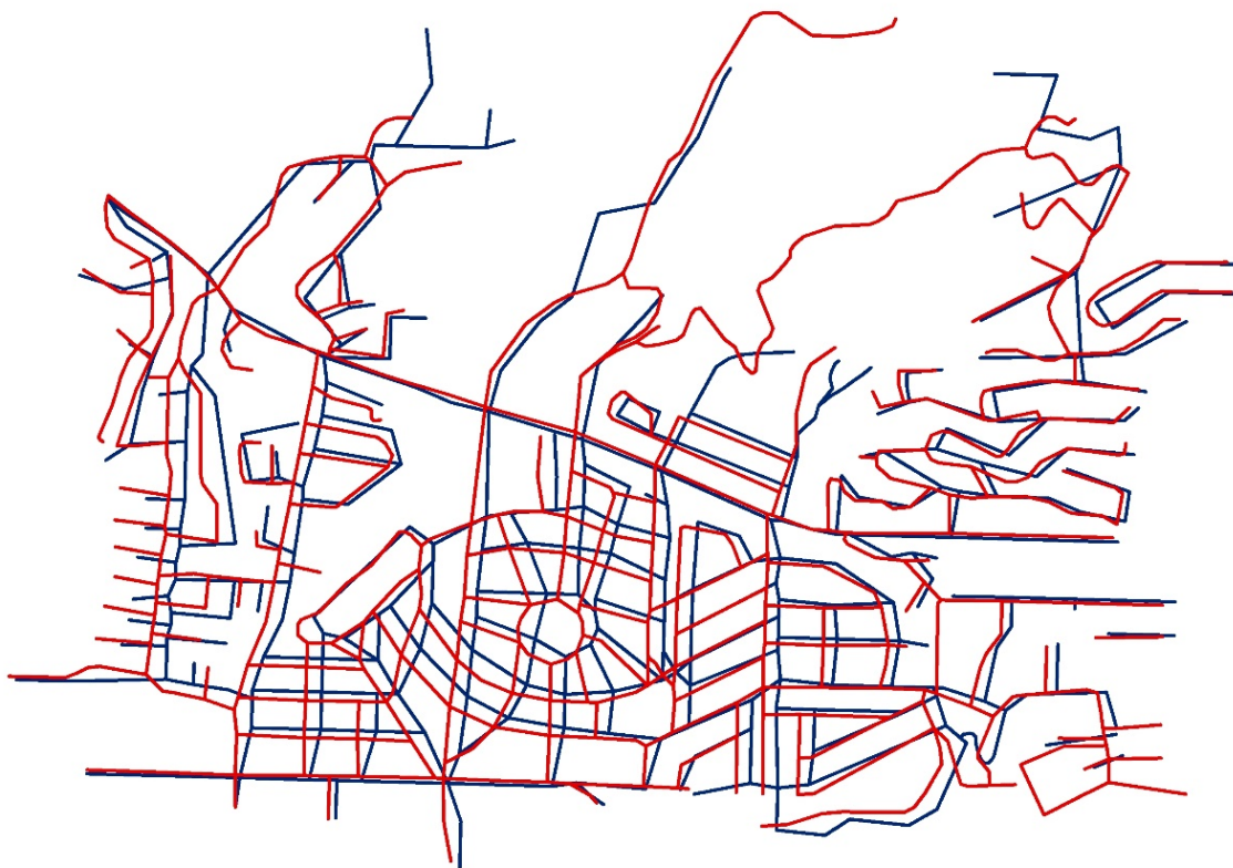
Figure 1. Positional uncertainty: Street networks in Santa Barbara, CA from two different data sources (Li & Goodchild, 2011).
