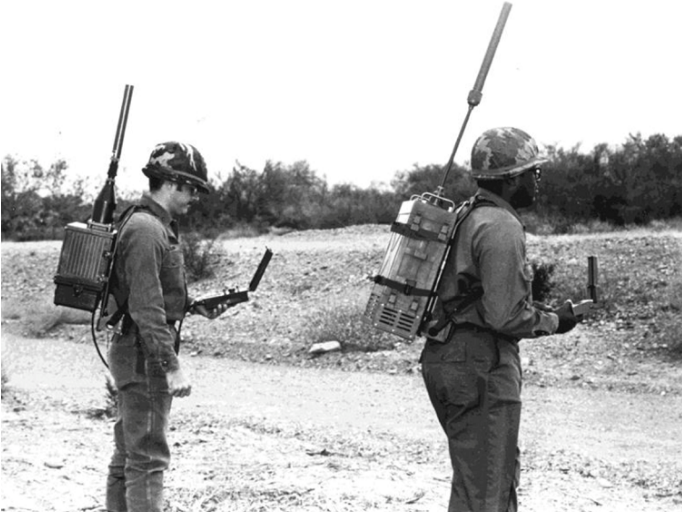
Figure 1. GPS receivers used by the United States military circa 1978. Source: https://bit.ly/2TS41Xx
