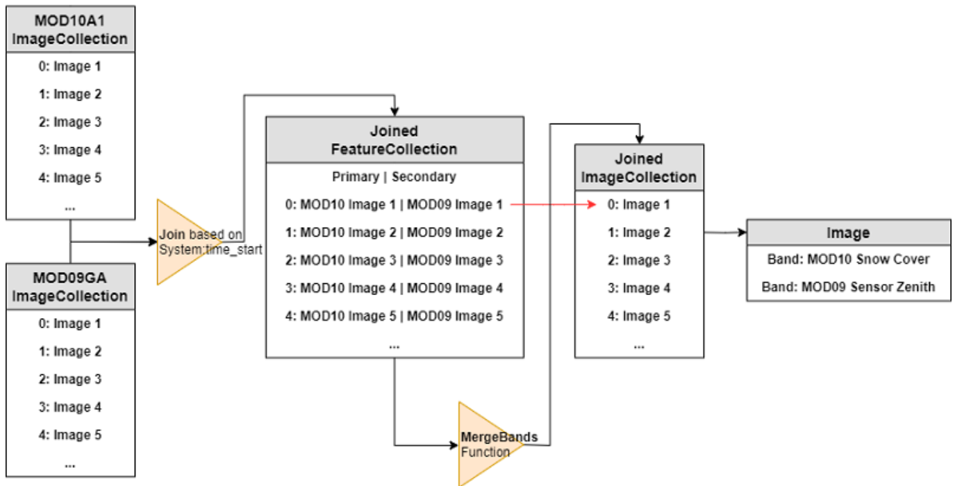
Figure 10. A visual representation of the MergeBands function we need to write to transform the results of our join into a more usable form. Source: authors.
