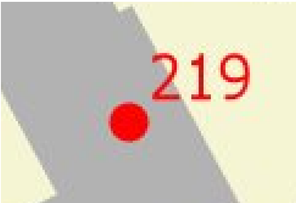
Figure 2: A JPEG using 85% compression, a medium-quality compression amount, of the same vector-based map shown in Figure 1. File size 18.3 kilobytes. Image magnified 400% from source image of 96-DPI. The image shows strong visual artifacts caused by the sharp color transitions in the image and is larger in size than the 8-bit PNG. Source: author.
