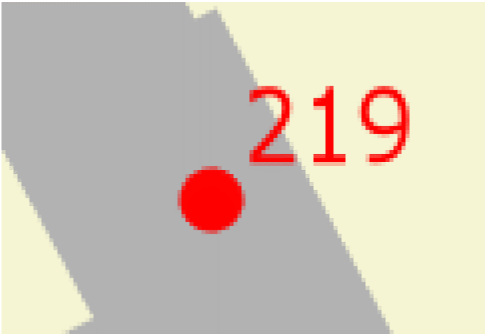
Figure 1: An 8-bit PNG of a vector-based map. File size 3.6 kilobytes. Image magnified 400% from source image of 96-DPI. The image has smooth transitions between colors from anti-aliasing but no visual artifacts. Source: author.
