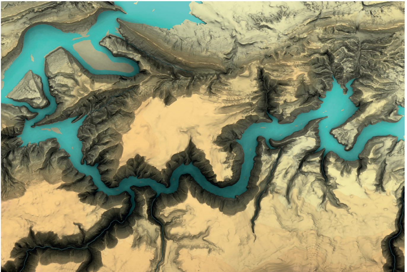
Figure 5. A map of the Flaming Gorge reservoir using hypsometric tints and shaded with an overcast sky model using the techniques described in Kennelly and Stewart (2014). Reprinted from Kennelly and Stewart (2015) with permission.
