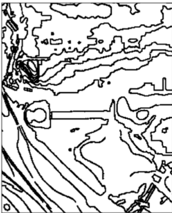
A part of the Washington West, D.C., 1:24,000-scale DLG showing hypsography (terrain relief).
