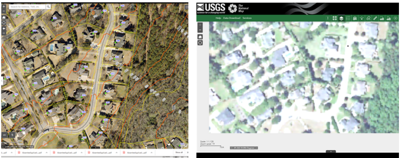
Figure 22. Comparison of 6-inch aerial imagery with 1-meter USDA NAIP imagery in Lexington County, South Carolina. Image sources: Lexington County GIS and USGS.
