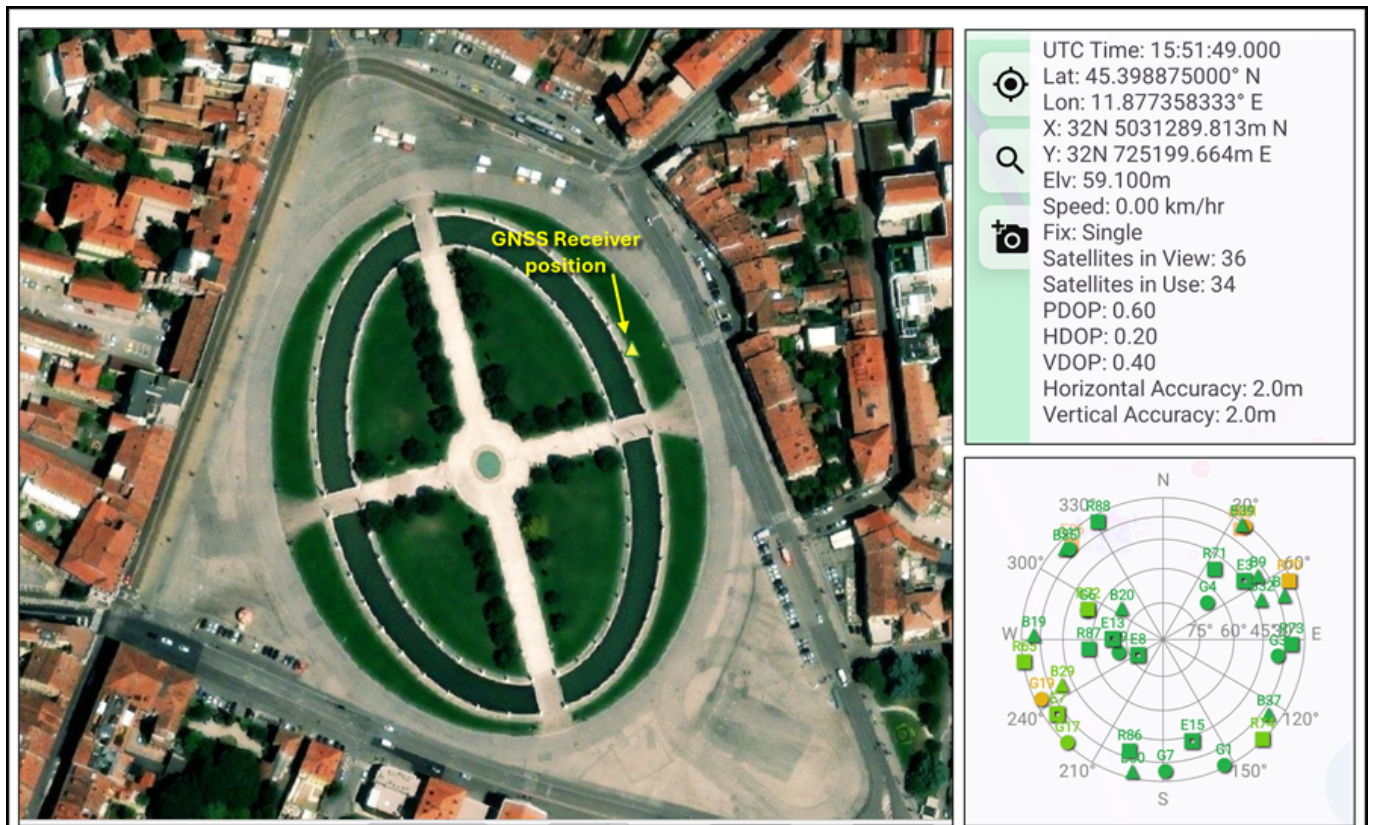
Figure 10. Observed satellite positions in the hemisphere above a cellphone-based GNSS receiver in the Prato della Valle, Italy on 4 June 2025 in front of the Galileo Galilei statue. The satellite in view and used in the position fix along with PDOP, HDOP, and VDOP estimates are all very good. Source: author.
