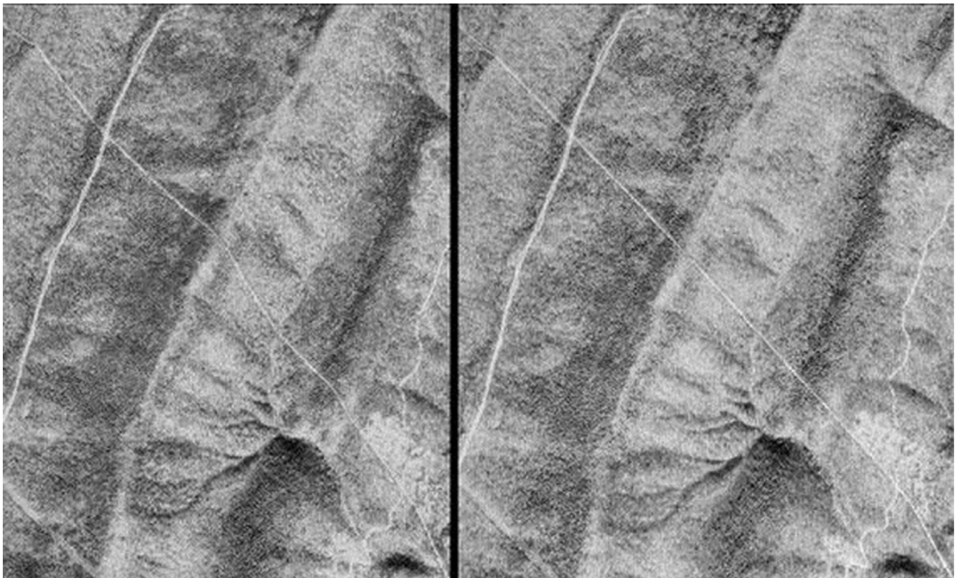
Figure 4. A pipeline extending southeast to northwest across the aerial photograph (left) appears to have curves as the result of terrain variation. In the digital orthophoto (right) the pipeline is seen in its true state as a straight line. Source: United States Geological Survey.
