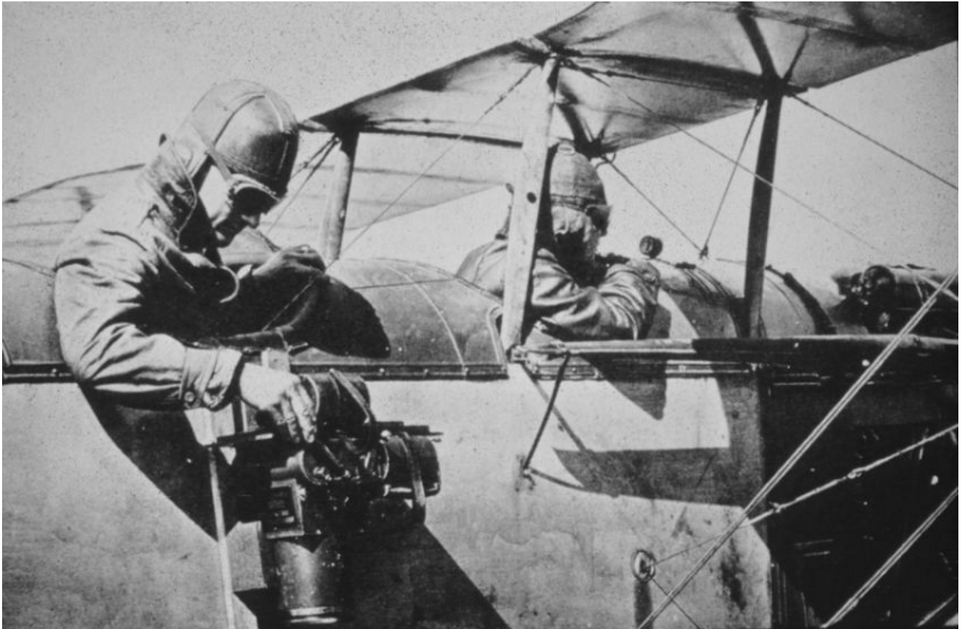
Figure 2. Reconnaissance aircraft used during World War I, with the pilot trying to maintain a level plane so that the photographer could take vertical photographs circa 1919. Source: United States Air Force.
