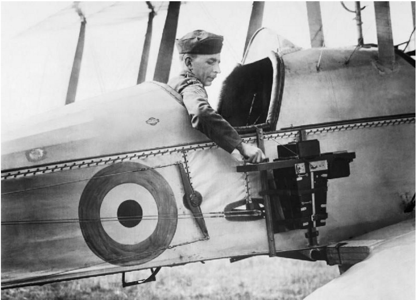
Figure 4: A B.E.2c reconnaissance aircraft of the RFC (Royal Flying Corps) with an aerial reconnaissance camera fixed to the side of the fuselage, 1916. Source: Wikimedia Commons.
