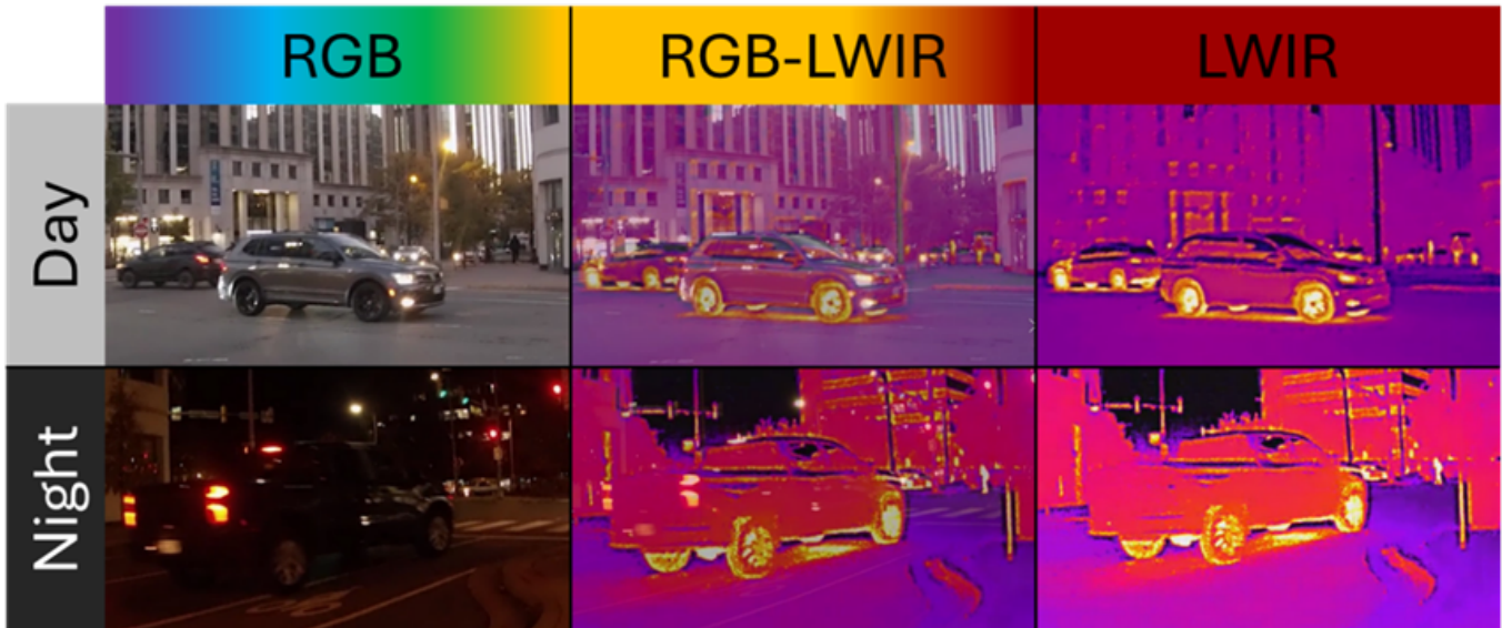
Figure 2. A comparison of RGB, RGB-LWIR, and LWIR images and the unique edges that each sensor extracts. Source: authors.
