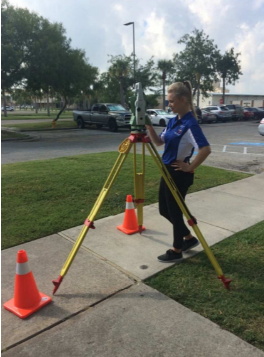
Figure 1. Surveyor using a Total Station. Source: author.
