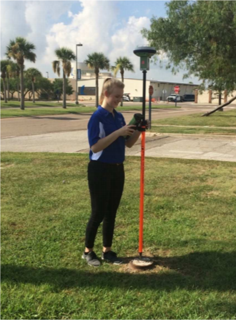
Figure 2. Surveyor using a Geodetic GPS Receiver and Data Logger
