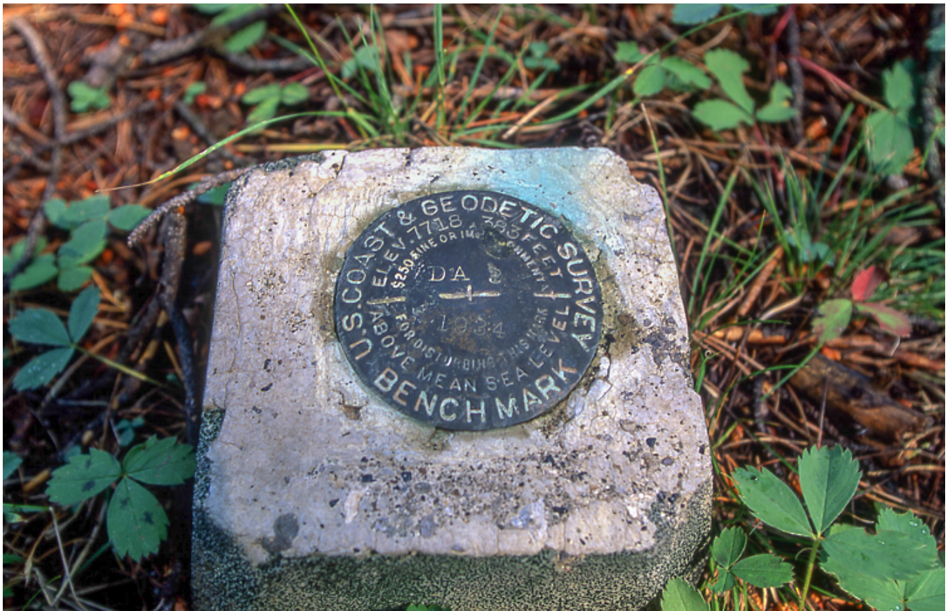
Figure 6. A benchmark established by the U.S. Coast and Geodetic Survey. Source: National Park Service - Jim Peaco . Used with permission.
