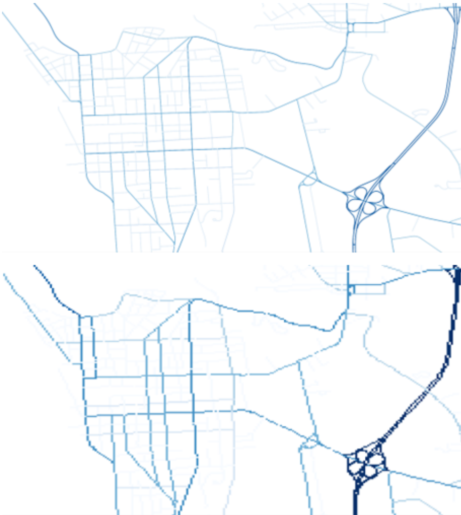
Figure 2. A linear street network symbolized via functional class specification depicted in vector format (top) with results from raster conversion (bottom). Source: author.
