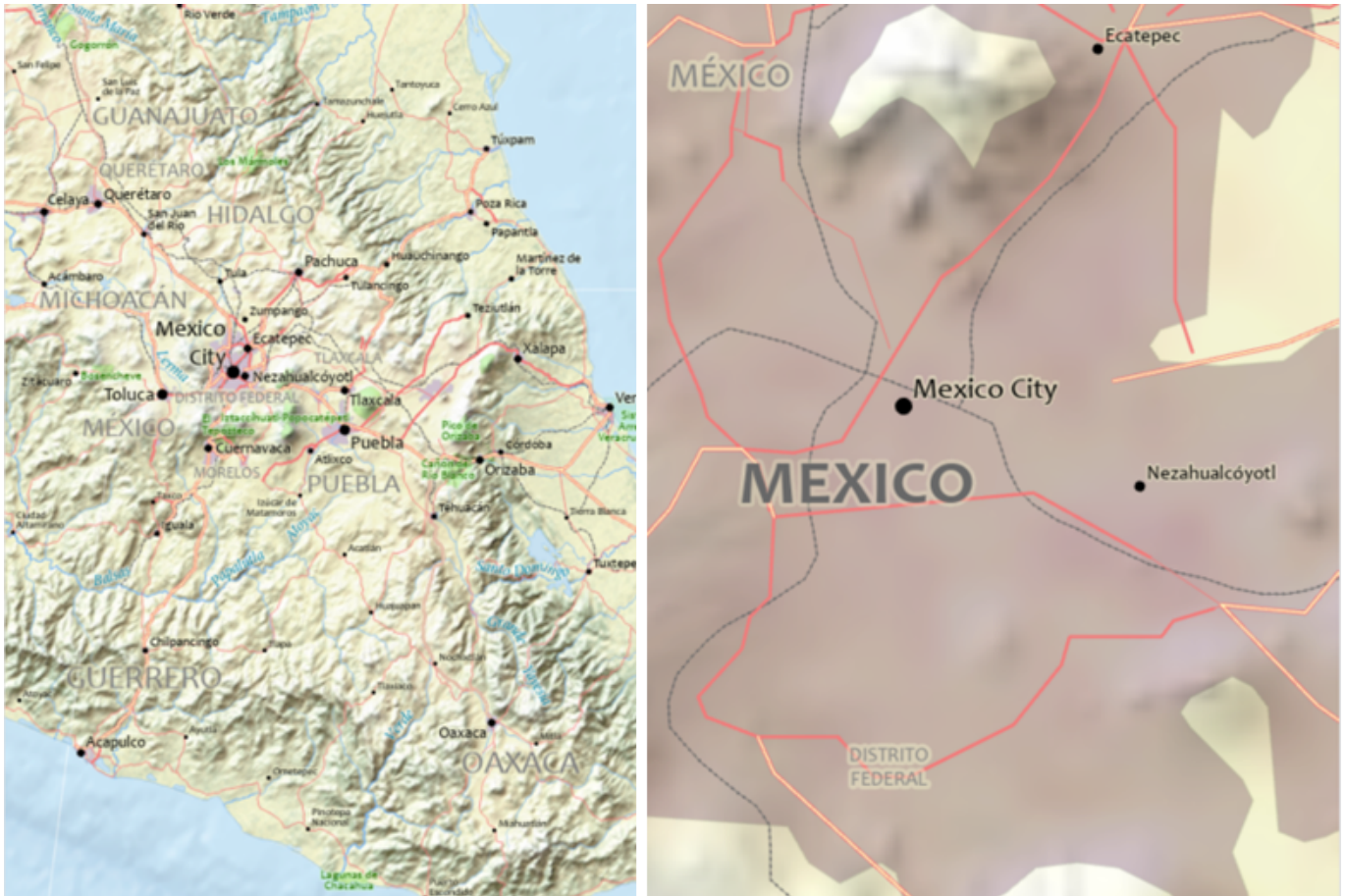
Figure 1. Data from Natural Earth ( naturalearthdata.com ), illustrating the concept of fitness for use and the relativity of data quality. Natural Earth is widely recognized as an excellent source for small-scale maps (left), but is entirely inadequate for street-level navigation (right). Source: author.
